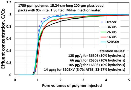
Figure 4—Polymer retention on illite using Milne injection water.
