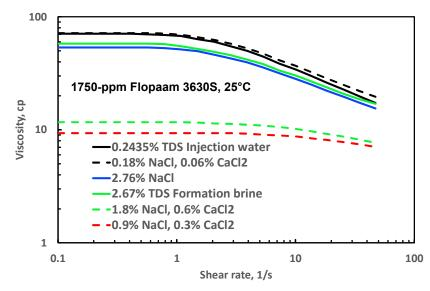
Figure 3—Viscosity versus shear rate for HPAM in various brines.
