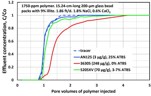
Figure 5-Effect of ATBS content on polymer retention with a hard brine.
