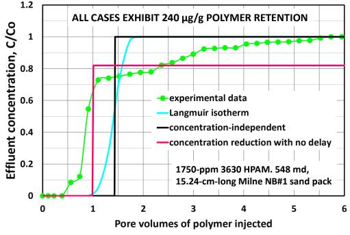
Figure 1—Various forms of the polymer retention function.
