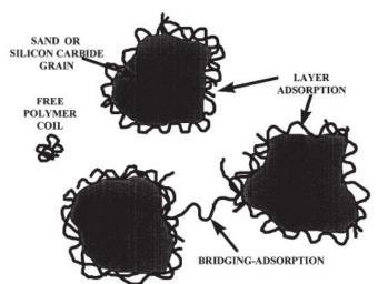
Figure 8—Illustration of the bridging-adsorption mechanism (from Zitha and Botermans 1998).
