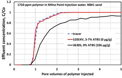
Figure 6—A small amount of ATBS reduces polymer retention in NB#1 sand.
