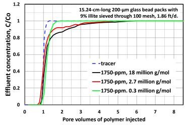
Figure 10—Tailing phenomenon in 9% illite versus flooding rate. Data from Seright and Wang (2022).
